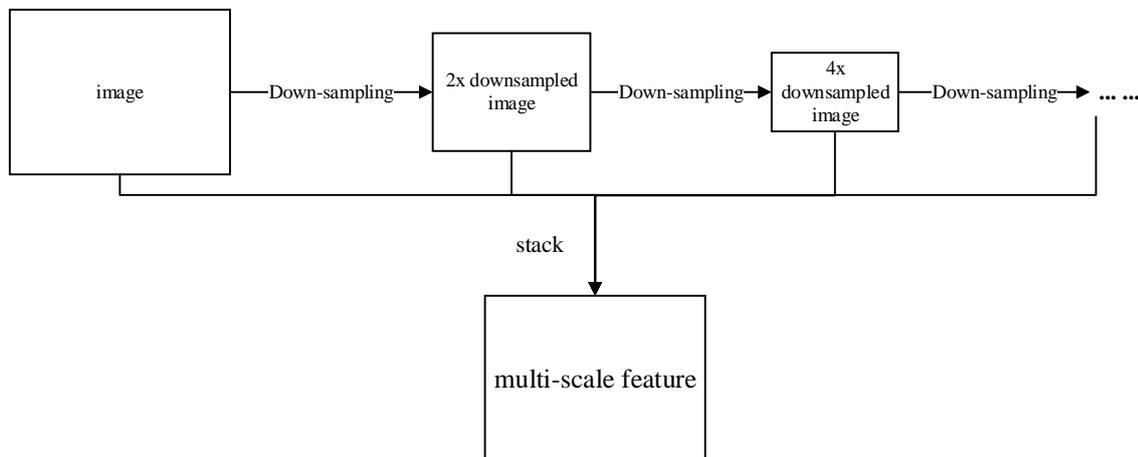
Figure 2. Process of multi-scale feature generation
